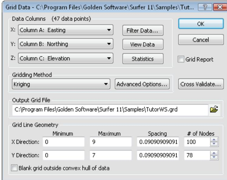
*The **Grid Data** dialog controls the options for gridding a data set. Set the Gridding Method, Advanced Options, Grid Line Geometry, and specify a Output Grid File name in the dialog before clicking OK. If the Grid Report box is checked, a report window will appear with information about the gridding process.*
