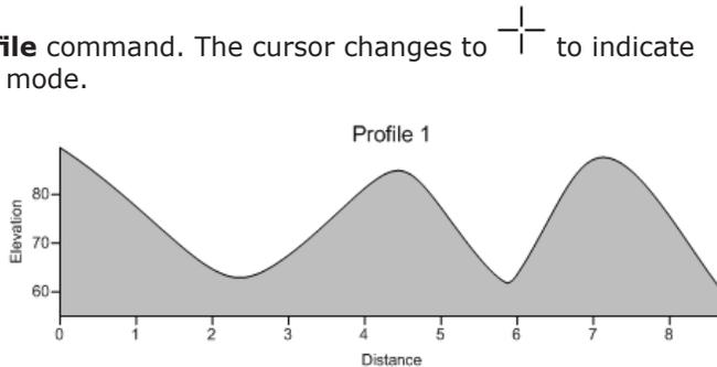
*The profile graph showing the elevation change across the drawn line is automatically created when the line is completed.*
